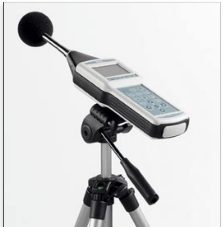
DL5 Noise Studio: Railway traffic module: 24-hour analysis with automatic transit search.
